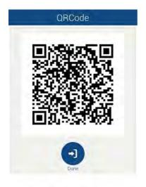
tap "done" once your camera LED rapidly blinks; ADS-446 & 456: Hold your mobile device approximately 4" to 6" (100mm to 150mm) in front of the camera lens to scan the QR code. When you hear a short beep beep sound, tap "Done" to finish.
