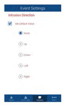
For example, if someone is entering the cameras view from the left and moving to the right, you would select the "Right" direction value for an intrusion to be detected. Please note; if motion detection is enabled, intrusion detection will not function correctly. Any movement will be detected as motion and a motion event will be created.
