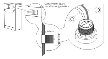
The push button can be installed on the top or front panel of a furniture WC unit in a variety of positions. Check for obstructions before cutting any panels.
