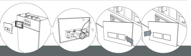
Cut aperture 172 mm x 105mm. Check for obstructions before cutting. Screw mounting bracket to the unit
