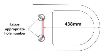
Once the 438mm dimension shown above is met and the template is parallel to the back edge, insert the bolts then tighten using a screw driver.
