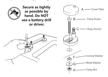
Remeasure the distance, making sure the 438mm dimension is met and remove the template and add the cover cap.
