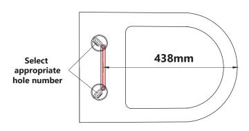
2 Once the 438mm dimension shown above is met and the template is parallel to the back edge, insert the bolts and tighten the underfix components, then tighten using a screw driver.
