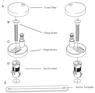
Note - alternative nuts and washers are supplied if you wish to secure the seat from underneath the deck of the toilet pan. If so dispose of the top fix inserts and tighten with the fixing key supplied.
