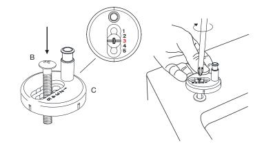
3 Using the anchor template provided, place over the two pins, making sure the template is parallel to the back of the pan.
