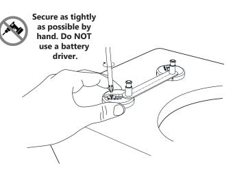
A Remeasure the distance, making sure the 430mm dimension is met and remove the template and add the cover cap.
