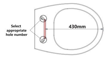
3 Once the 430mm dimension shown above is met and the template is parallel to the back edge, insert the bolts then tighten using a screw driver.
