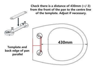
Once the template is in place and correctly positioned (430mm +/- 3 from the front of the pan to centre line of the template), hold the hinges securely and tighten the fixing screws with a screw driver. Remove the template.
