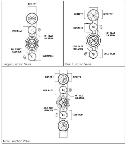
3. Connect the outlet pipework to the chosen shower accessory (wall elbow, shower head, etc.) and turn on the water supply to check for leaks.
