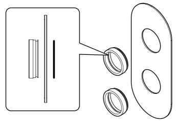
7. Apply a small bead of silicone on the outer edge of the back of the cover plate. Slide the cover plate and trim rings over the valve body up to the finished wall surface, covering the hole. Allow the silicone to fully cure before using the shower system.
