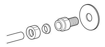
Thread the cover plate onto the threaded connector.
