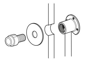
From the back surface of the wall plate there should be approximately 32.5mm of thread to make your plumbing connection through the finished wall surface.
