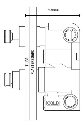
2. With the valve securely mounted, make the appropriate plumbing connections to the hot and cold supplies with PTFE tape. The hot and cold inlets are marked on the valve for easy identification.
