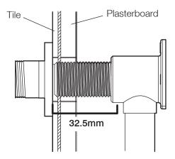
With the compression fitting and the compression nut positioned on the shower arm, insert the arm into the threaded connector. Tighten the compression nut onto the threaded connector until the arm is held firmly in place.
