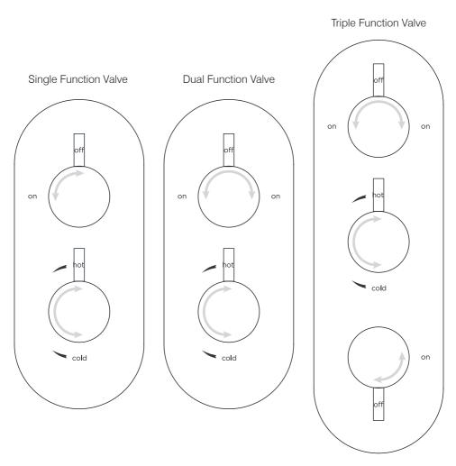
Rotating an outlet selection handle to an 'ON' positions will select the outlet plumbed into that position on the valve. Returning the handle to the 'OFF' position will turn off the water supply to the outlets. For three function valves, the outlet plumbed into the single function control can be used at the same time as one of the other two functions.
