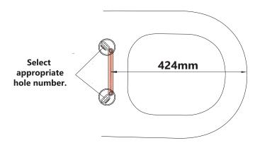
Once the 424mm dimension shown above is met and the template is parallel to the back edge, insert the bolts then tighten using a screw driver.
