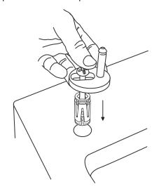
Place the template over the anchor pins, selecting the appropriate hole numbers (on the anchors) so that the 424mm dimension from the front of the pan to the centre line of the template is met.
