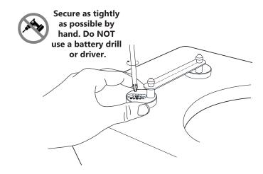
Remeasure the distance, making sure the 424mm dimension is met and remove the template and add the cover cap.
