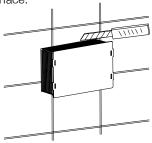
2. Screw the fixing arms (supplied in the box) onto the cistern. The rods may need cutting down depending on the thickness of the finished wall/surface.
