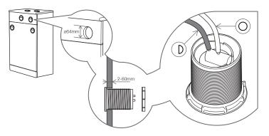
The push button can be installed on the top or front panel of a furniture WC unit in a variety of positions. Check for obstructions before cutting any panels.
