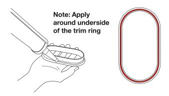
5 Insert the trim ring into the front side of the fascia. Wipe away any excess silicone around the trim ring.
